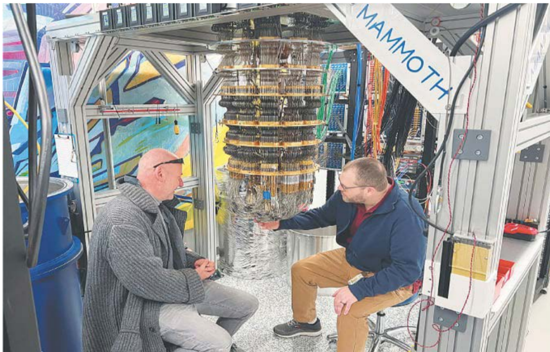
GOOGLE Quantum AI's Hartmut Neven (left) and Anthony Megrant (right) examine a cryostat refrigerator for cooling quantum computing chips at Google's Quantum AI lab in Santa Barbara.
